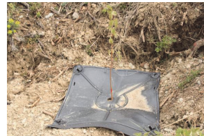
New biopolymer-based semi-rigid plate, 100% biodegradable (DTC)
