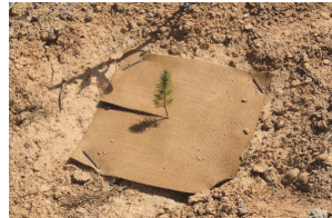
Woven jute cloth treated with furan bio-based resin for increased lifetime, 100% biodegradable (La Zeloise)
