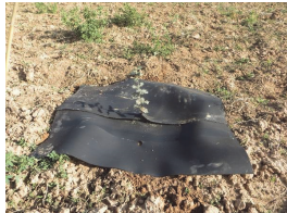
Recycled rubber based mulch anti-UV, reusable in successive tree plantations. 1.5 mm thick (EcoRub)
