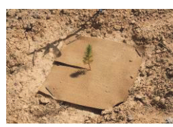
Woven jute cloth treated with furan bio-based resin for increased lifetime, 100% biodegradable (La Zeloise)
