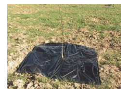
Black new biopolymer-based frame, 100% biodegradable, fused to a commercially available black biodegradable film (DTC)
