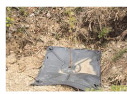
Black new biopolymer-based semi-rigid plate, 100% biodegradable (DTC)
