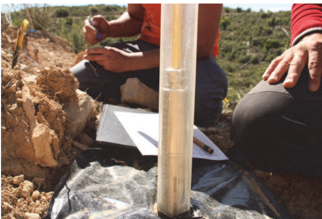
Soil moisture measurement equipment: IMKO TDR probe with reading device; different moments of soil moisture measurement at two depths
