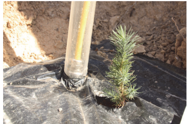
Soil moisture measurement equipment: IMKO TDR probe with reading device; different moments of soil moisture measurement at two depths
