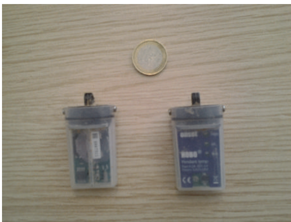
Soil temperature equipment: HOBO Pendant thermometer; datalogger built-in
